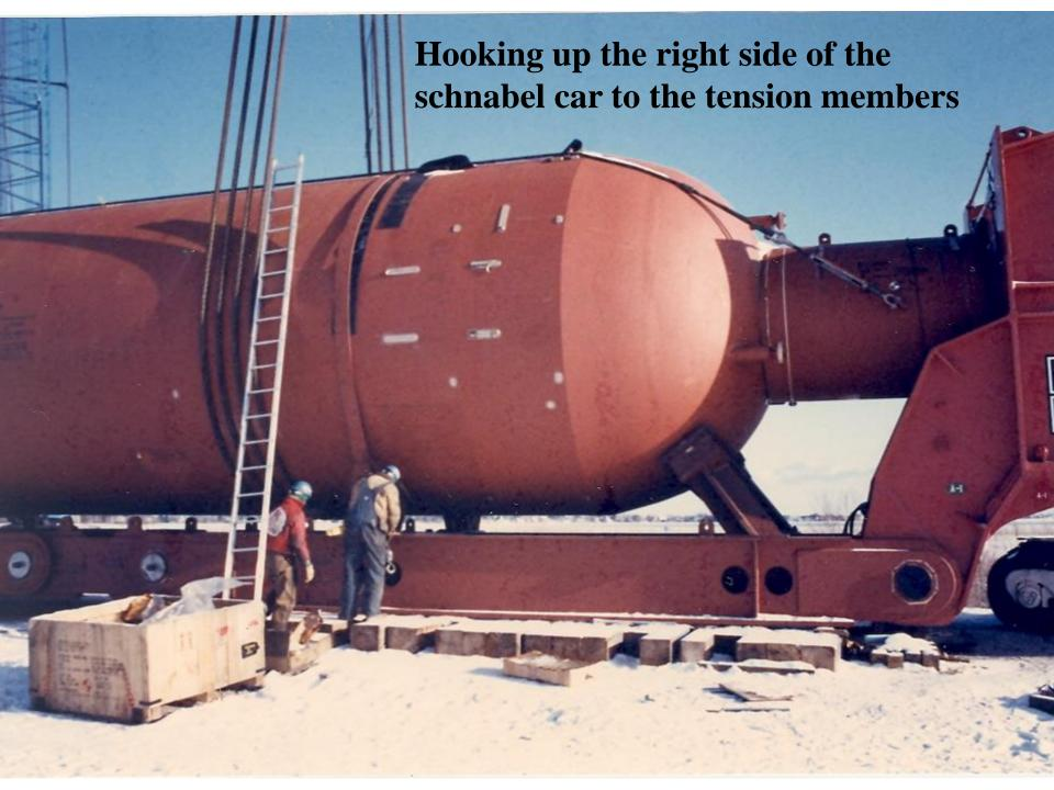
Adjusting the height of the tension members Above The Rails. The Goal is 24'' ATR
